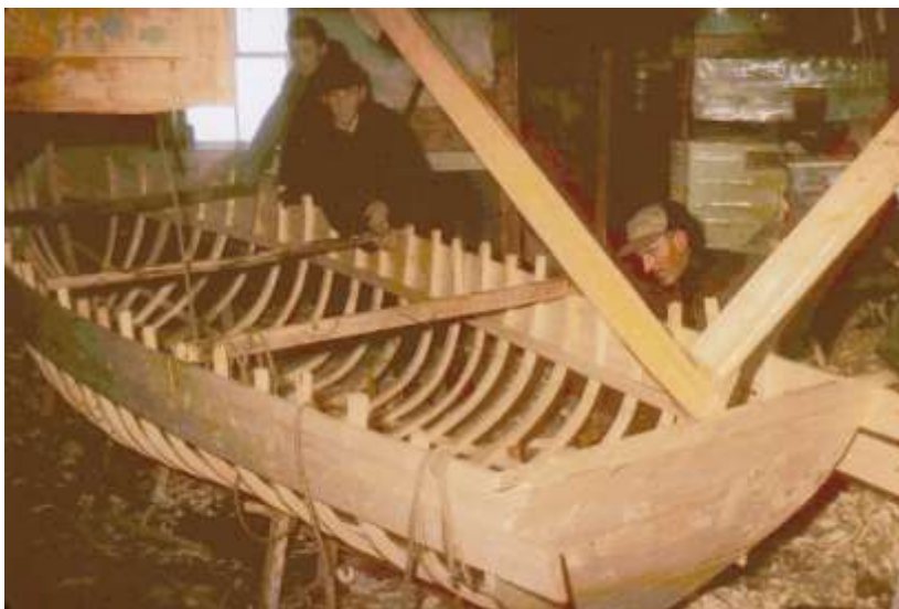
Figure 8 Gilbert Simms building a punt, with Gerald Pilgrim and Herbert Simms looking on.
