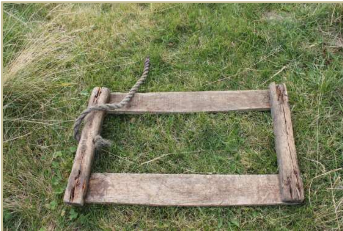
Trawl tub sleigh used on the stage to haul a trawl tub full of salt-water
