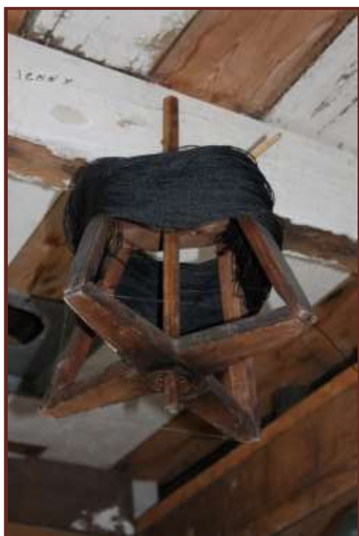
A twine jenny, which operated like a large spool and was suspended from the ceiling. Fishermen knitted theirs nets in the evening, so the twine jenny (or spin-me-jenny) was usually in the kitchen.
