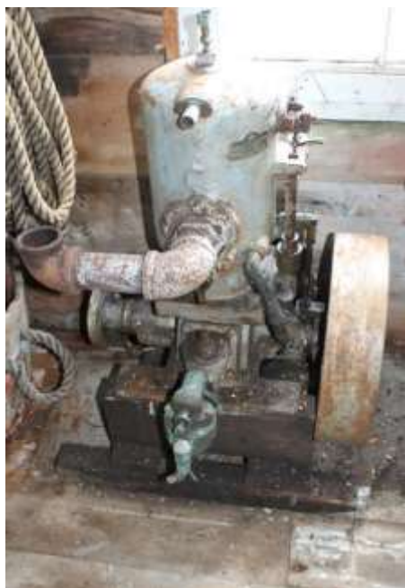
8Hp make and break engine. Photo, Kathleen Tucker
