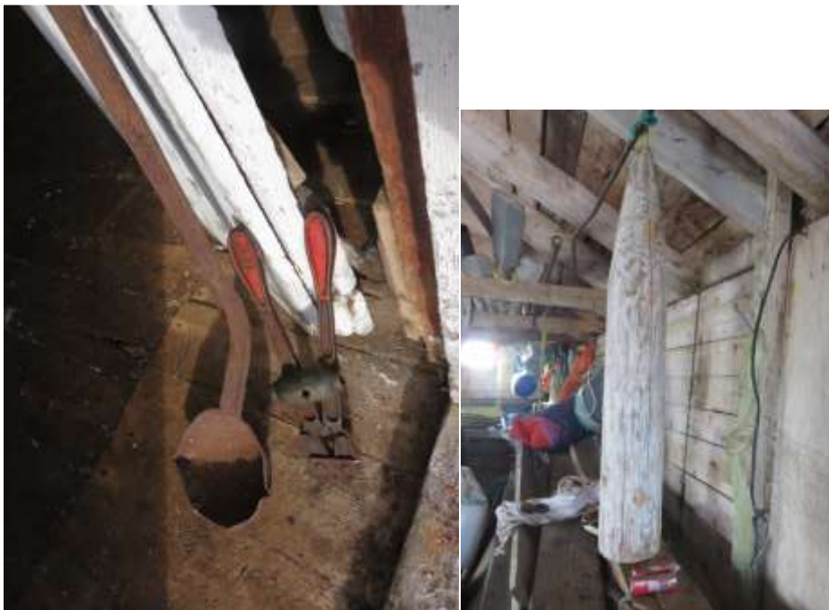
Looking down on a ladle and mold used for making lead balls for a trap (left). And (right) a watch buoy used on the end of a grapelin.
