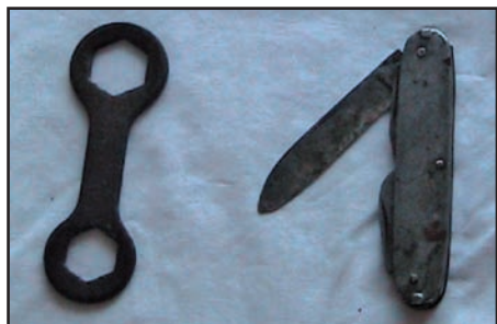
Figure 7 Scythe Wrench (left) used for changing the size of blade on a scythe. A pocketknife was a fisherman’s pocket companion.
