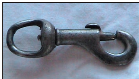
Figure 6 Dog snap for attaching a dog to a line.
