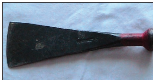
Figure 2 Caulking Iron for tapping oakum into the seams of a boat.
