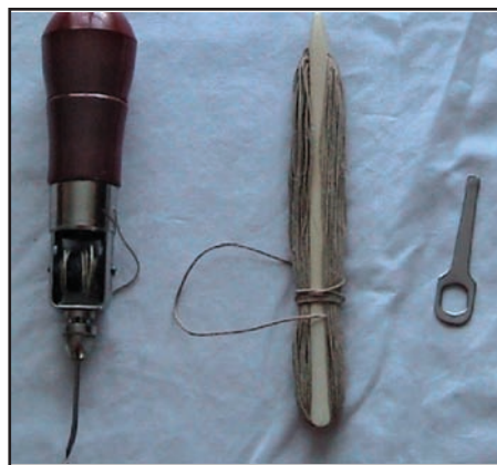
Figure 9 Awl Tool for sewing sealskin boots
