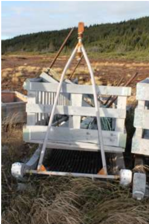
Figure 95 A komatik with a piece of truck box liner affixed to the runners.
