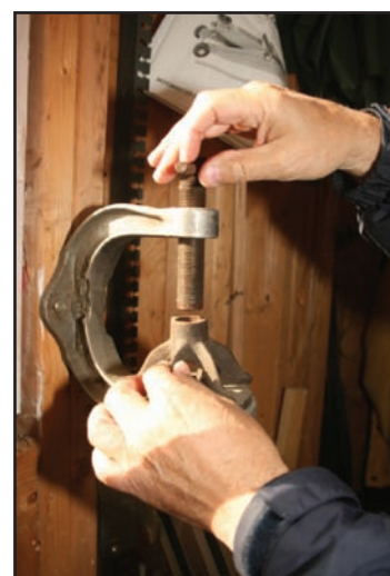
Figure 6 The hot patch machine was used for patching inner tubes
